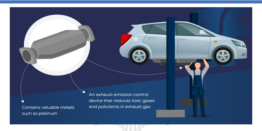
Catalytic converters help clean your car's exhaust emissions using chemical reactions with precious metals like Platinum, Rhodium and Palladium.
